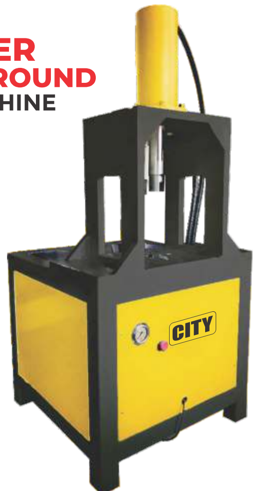
HYDRAULIC SINGLE CYLINDER PIPE CUTTING MACHINE (30 TON)
